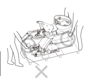
Do not make scratch or damage the floor while moving the unit. Please use the carriage jig to move it.
