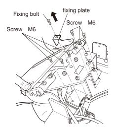
2. Remove the fixing bolt for carriage.
