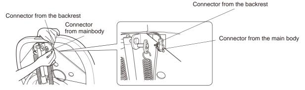
2. Fix the connector on the hook as the following figure shows.
