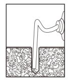
2.Clean each anchor hole thoroughly using a vacuum cleaner, with a narrow nozzle attachment to reach into the hole and remove all debris.
