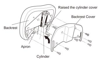
2. Attach the backrest cover and fixed with six screws(M4 x 18)
