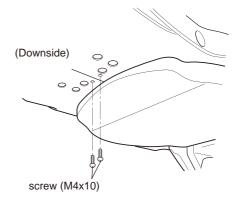
Note: In attaching the seat cover, the apron to be put on the seat cover as the figure shows.
